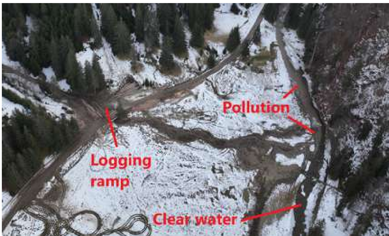
Figure 34: aerial photo of logging ramp showing muddy, polluted runoff spilling into Valsan River, taken in February 2023.
