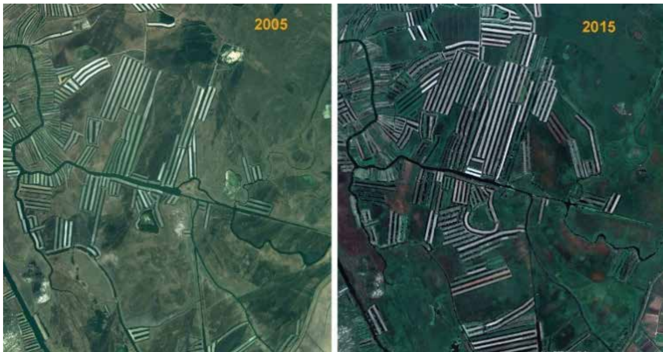
Fig. 14: Drainage and melioration of wetlands for the cultivation of tangerines and other fruits in the Croatian part of the Neretva Delta (Google Earth 2019).
