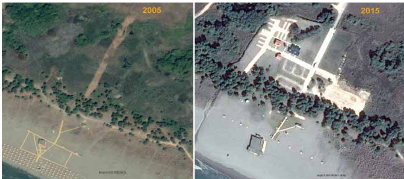
Fig. 6: The development of beach infrastructure along Velika Plaža, Montenegro, destroys coastal swamps (locally known as knetas). In addition, the reduction of the sediment load of the Bojana-Buna River drives the regression of shoreline through erosion (Google Earth 2019).
