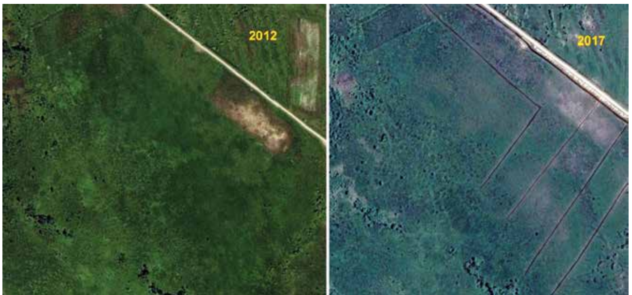
Fig. 21: Construction of new drainage ditches to gain arable land in Livanjsko Polje (Google Earth 2019).
